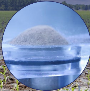
S28 - Core sample being eroded by water flow
